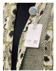
The badges work in several ways. The button will be pressed three times if assistance is needed in a classroom or work space. The badges have a built-in GPS that identifies the location and allows for a quick response by the school and then district wide. For more serious situations such as a dangerous person in a school or work location, the button is pressed 8 times and the building will be put on immediate lockdown.
